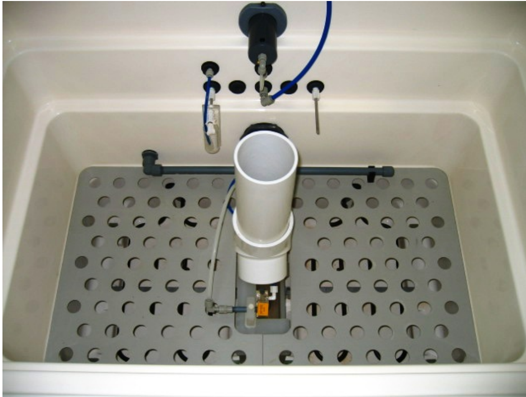
Photograph 6 Cyclic Corrosion Test Chamber
